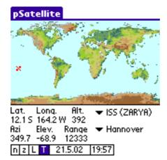
The top half of the Main display has the world map and will show indicators (bitmaps) for the satellite and the (observers) tracking location.
